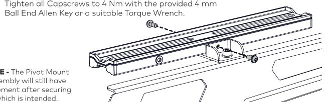
**NOTE -** The Pivot Mount assembly will still have movement after securing which is intended.
