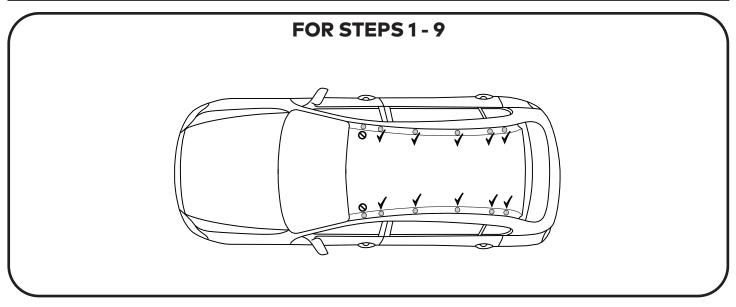
Using a stanley knife, carefully scrape away the paint seals to expose mounting holes.
