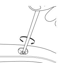
Note: Apply upwards pressure to the rail to prevent the captive nut from dropping and spinning while the bolt is being undone.
