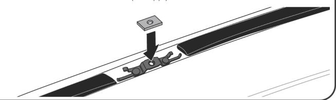
ASSEMBLE PIVOT BRACKET TO RUGGEDLINE
