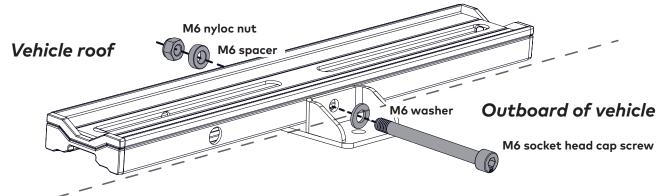
Secure with the M6 socket head cap screw and M6 washer (outboard of vehicle) and M6 spacer and M6 nyloc nut (inboard of vehicle) from this kit **in the order as shown.**
