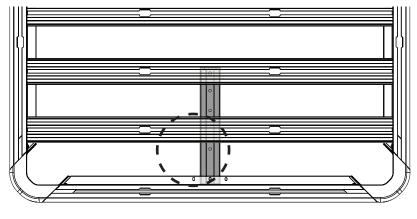
Loosen the three M8 nuts along the centre support and remove the single M6 button head cap screw. Reinstall the M6 button head cap screw in the desired location and retighten all M8 nuts to 7 Nm and the M6 button head cap screw to 4 Nm.
