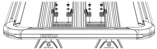
NOTE - Do not to over tighten slat clamps past 7 Nm as this may reduce clamping force.
