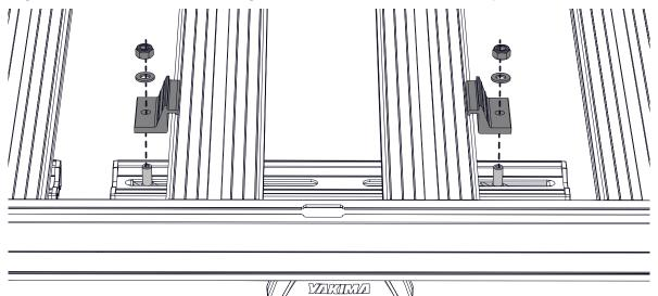
NOTE - Do not to over tighten slat clamps past 7 Nm as this may reduce clamping force.
